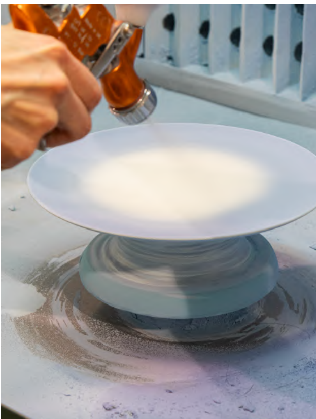
Enamelling of a plate
