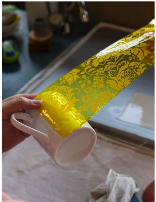
Placing the Chardons decal on a cup
