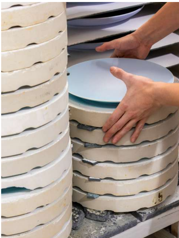
Placing parts in the kiln
