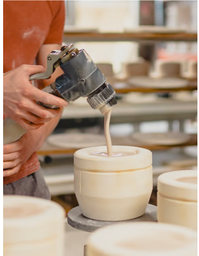
Pouring the liquide cast into a mould
