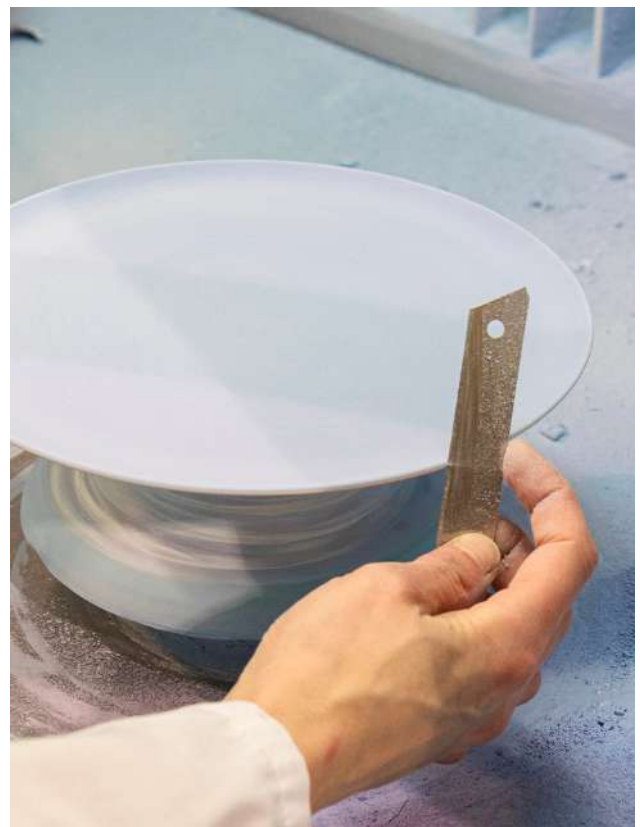
Hand finishing of an enamelled plate
